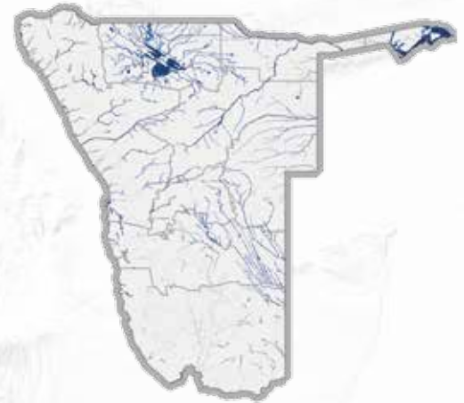
Flood hazard map for 1 in a 100 years probability evaluated under current climate conditions, the scale of blues represents different water depth values.
